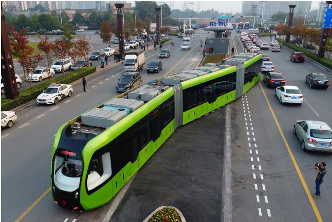
The battery-powered trackless tram, or ART, in operation in Zhuzhou, showing the trackless autonomous guidance system.
