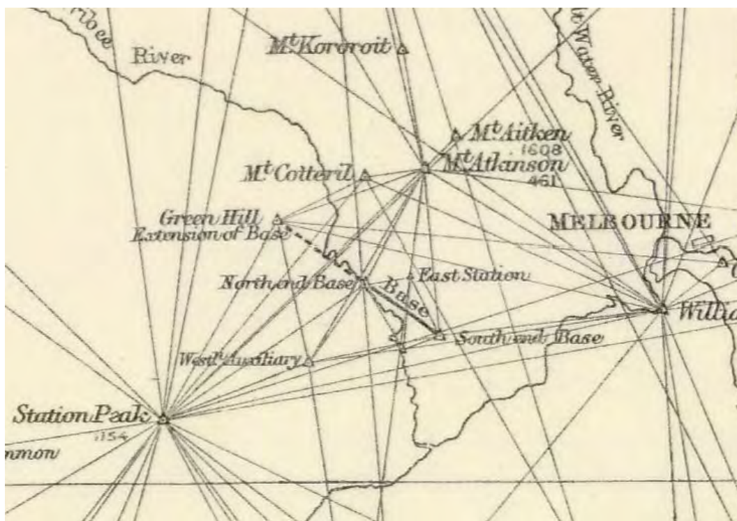
Figure 11 Detail of 'The triangulation of Victoria' map, c. 1870, with the Werribee base line shown Source: Department of Crown Lands and Survey, Victoria, State Library Victoria
